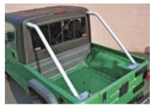
**24.** Now that the hardtop is completely installed, reinstall the rear cage tubing pieces. These will need to be painted black or painted to match the Jeep body color.
