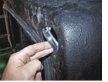
**21.** GR8TOPS can provide the optional rubber grommets to seal the hole in the hardtop where the tubing passes through. Move the top back past the tubing disconnects and install the two rubber grommets using a light amount of lithium grease or WD-40 to help when sliding the top back over the tubing joints.
