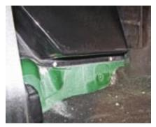
**15.** Lower the bulkhead into place. The bulkhead has a contoured molded ledge that conforms to the Unlimited's wheel wells and lower step ledge. Once the bulkhead is positioned, use the supplied self-tapping sheetmetal screws to install the bulkhead into place from inside the cab. There are four pre-drilled holes on the bottom and two on either wheel well location of the bulkhead. For standard short-wheelbase TJs, the bulkhead is a different shape, but the installation process is the same.
