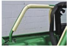
**6.** Separate and remove the hard shell foam pads from the rear cage pieces. Each piece has a plastic insert that is popped into place on the rear bars. Carefully remove the foam pieces from the inserts in the cage.
