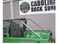
**12.** The completed cage provides better triangulation than the stock setup and offers many future options, such as a bed-mounted spare tire carrier or a Hi-Lift jack mount. Adding a front down the dash cage kit would also structurally enhance the factory cage.
