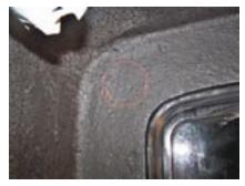
**18.** Using a grease pencil, mark circles on the inside of the hardtop on both the driver and passenger sides where the disconnects touch the top. These marks will be used for cutting the access holes to allow the cage to pass through the top. Ensure that the hardtop is sitting completely and firmly on the bedrails to guarantee that the hole markings are in the correct position.
