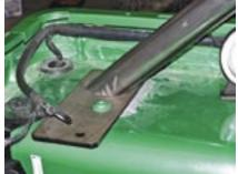
**11.** We solicited the qualified help of Carolina Rock Shop to fabricate two sets of new rear rollbar pieces using the GR8TOPS tubing disconnects. On the floor end, both sets had foot plates installed to mate to the existing rollbar mounting holes. One set was designed in the retro Scrambler/CJ look and the other used the OEM pieces we removed. This way we can actually reinstall the factory cage bars, the factory seat belts and rear seat if we ever want to return to the stock setup.
