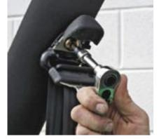
**4.** Using a T45 Torx bit, remove the rear shoulder seat belts. The upper shoulder mount bolt can be accessed by popping the plastic cover from the bottom edge. Remove the lower shoulder mount bolt by the rear cage foot and also on the inside of the lower wheel well. Remove the center floor seat belt receptacle and the two black rear seat brackets that are mounted to the floor.
