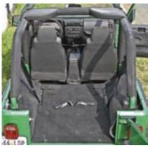
**1. & 2.** Remove the OEM soft top or hardtop and the existing frame and all hardware. The factory plastic soft top door surrounds must be removed as well. Remove the rear carpet (both the center floor piece and the two wheel well pieces). Flip the two front seats forward to give as much cab room as possible for the installation process.
