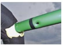
**8.** Measure 4.5 inches from inside the main hoop, along the rear cage bars on both sides. This tends to be just about centered between the speaker pod mounting bolt dimples. Mark this with a piece of tape all the way around the bar to serve as the cut marks for the rear bars.
