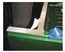
**16.** Install a layer of camper foam tape on the top ledge of the bulkhead and to the 5- to 6-inch stretch of Jeep body rail. This helps prevent scuffing and provides a good seal between the hardtop and the Jeep body.
